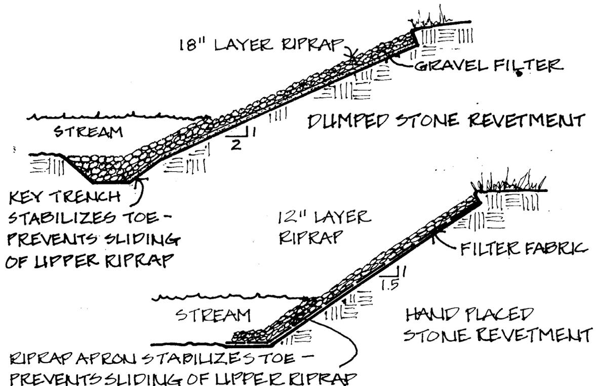
**Riprap revetment on a stream bank**
