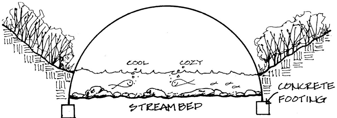
**Bottomless arch culvert to accommodate fish passage**
