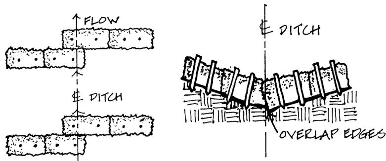
**Type B** – Use at the base of a slope or where the existing ground slopes away from the toe of the filled embankment.
