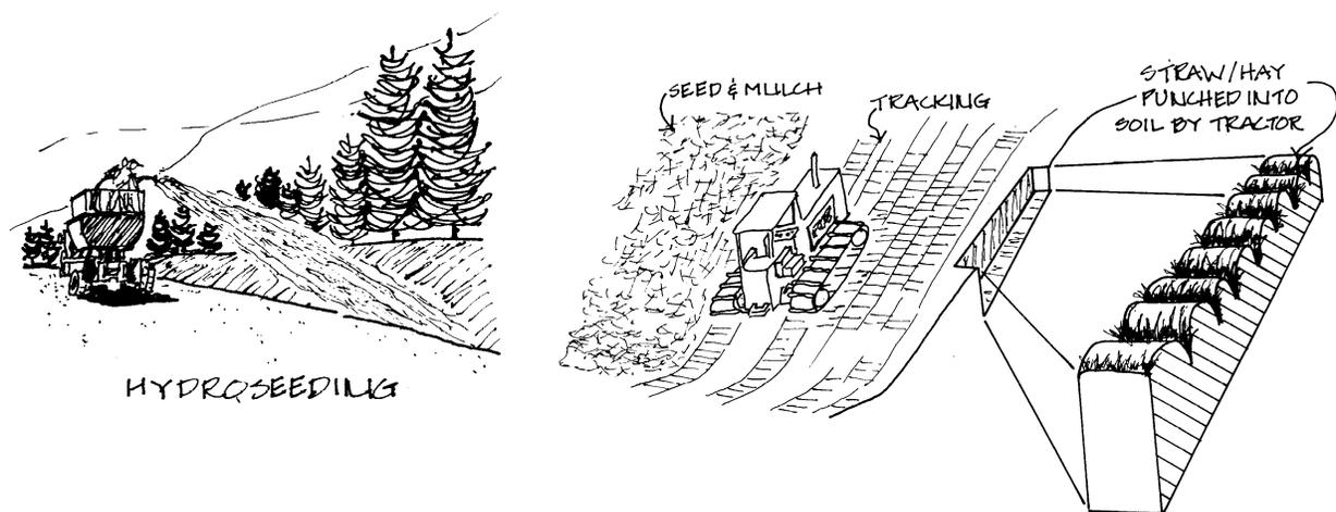
***Hydroseeding and surface roughening, two low cost ways to stabilize a slope***
