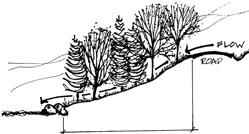
***Cross section of a filter zone***
